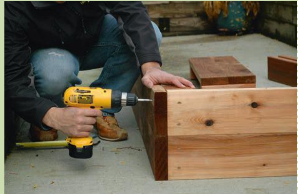
Assemble the frame by attaching the longer 2-by-6s to the short ends.
