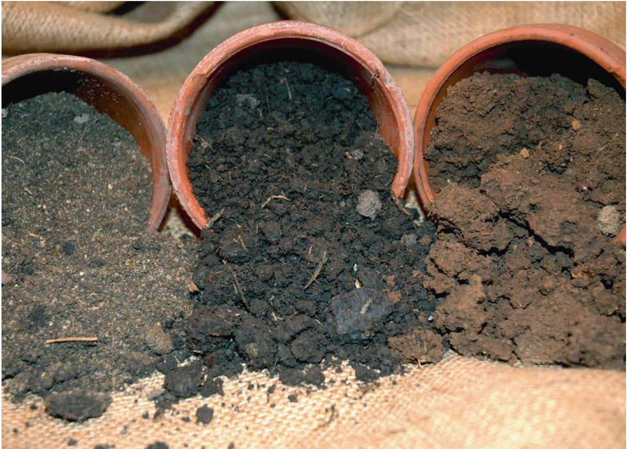
Example of sandy soil, loam, and clay soil (from left to right).
